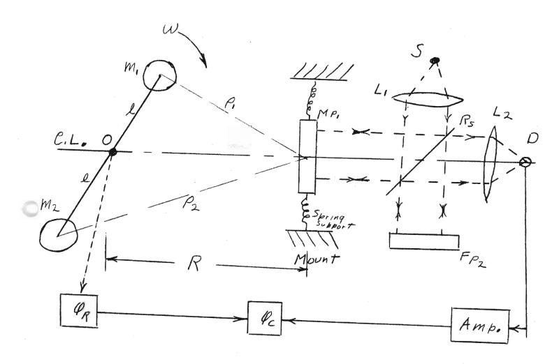
Figure I. Schematic of Proposed Experimental Setup.
