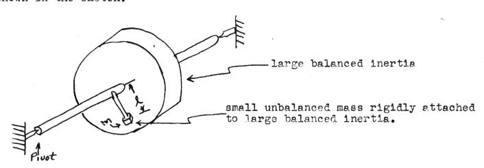
In what follows, we consider that the arm supporting the small mass m is initially lined up along the local vertical and ask if it is possible to adjust the three parameters available, I, l, and m such that this arm remains along the instantaneous local vertical regardless of any arbitrary horizontal acceleration normal to the pivot axis of the system.
